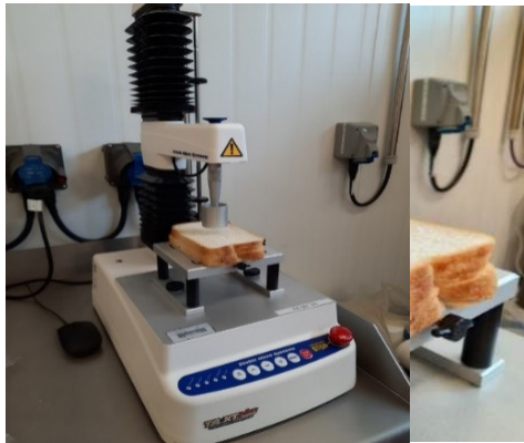
Figure 4.6. a) Texture Analyzer (TA.XT Plus, Stable Micro System, UK); b) 35 mm probe
